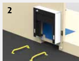
Telesco leveler covered by the sectional door for refrigerated warehouse. With open hatch.
