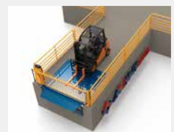
Protective barrier function to prevent that the forklifts could fall in the docks.
