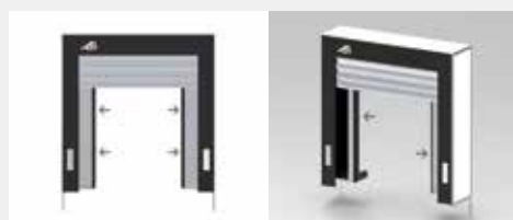
Option of removable additional reinforcement with velcro system.
