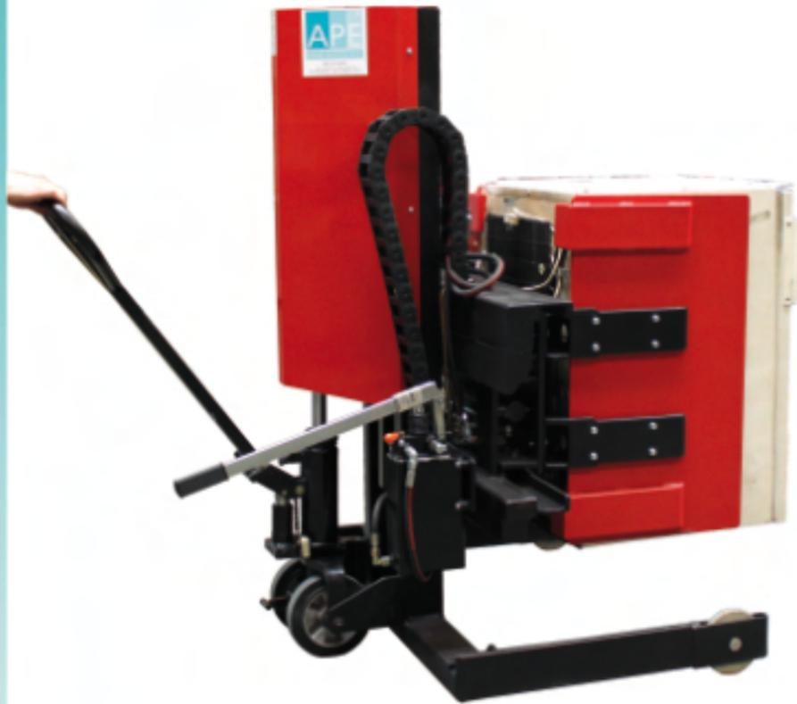
This grabber is constructed to lift and carry sensitive refrigerators from 45 cm to 110 cm of breadth.
