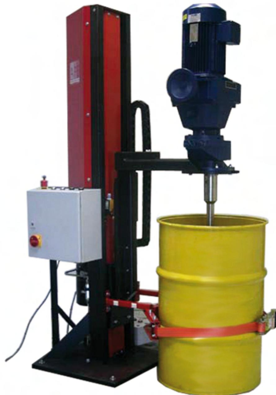
Agitators seem to have a very simple setup at first glance, but constructing them demands for careful construction work and safety design. The rotating stirring spindle holds great potential for danger. APE solutions for mixing are secure, easy and ergonomic to use.
