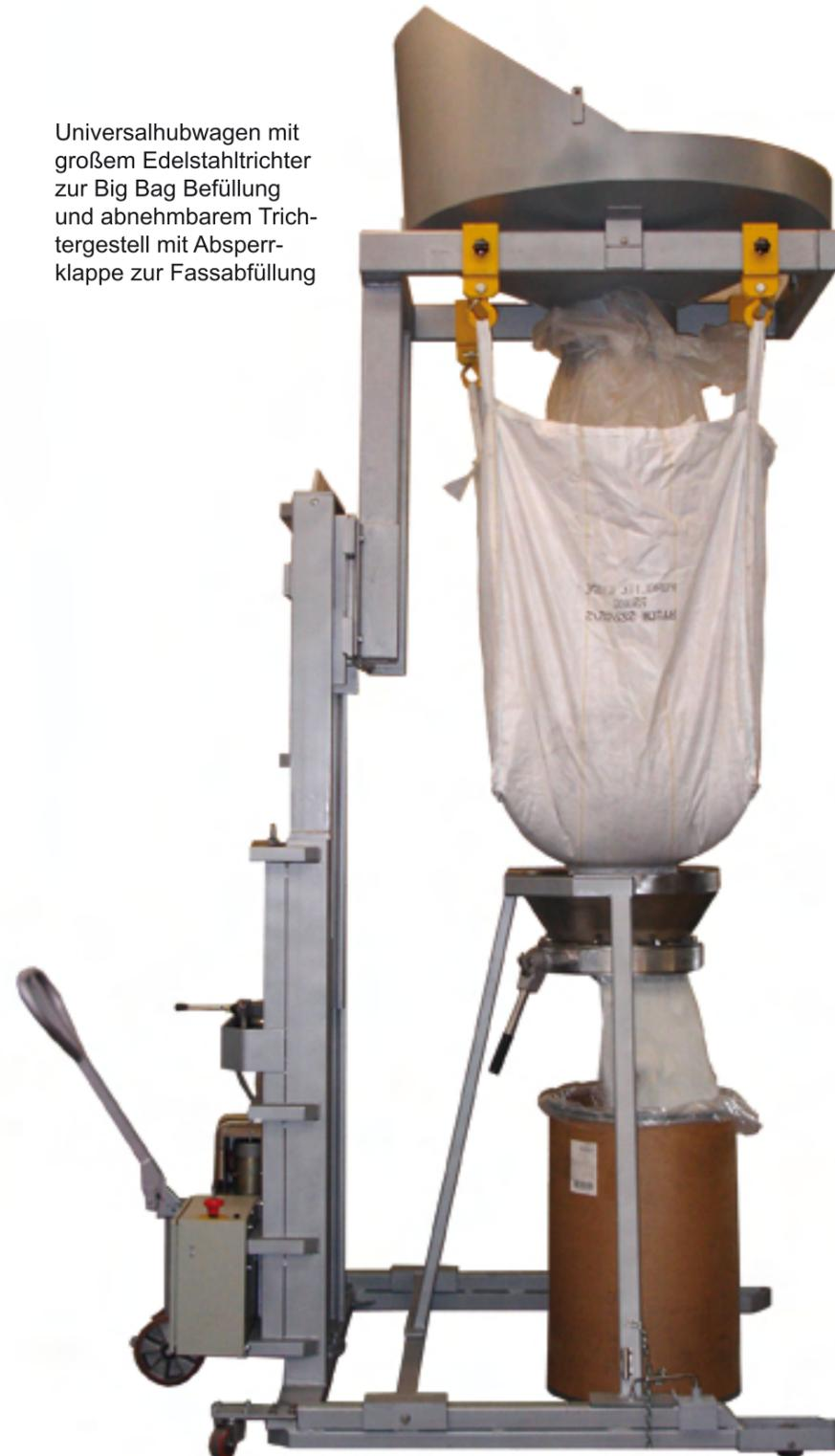
Universal stroke lift with big stainless steel hopper for filling of Big Bags including a removable hopper frame with the spear flap for barrel filling.
