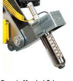
**Remote Mandrel Gripper Retraction Systems** Allows operator to stand behind machine to load and unload rolls
